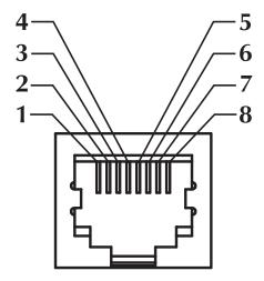
The figure above has the perspective looking into the printer RJ-45 modular connector.
